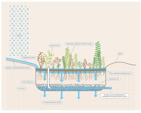
Figure 2. Illustration of a typical bioretention cell system
