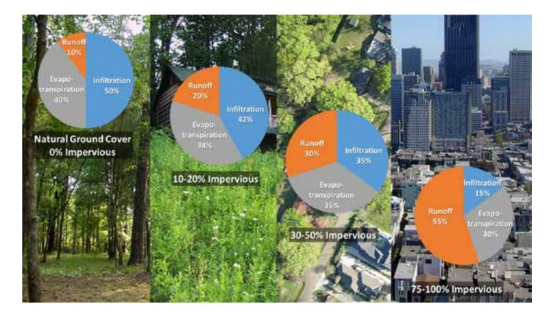
environments. By implementing a combination of techniques, GSI captures and treats stormwater runoff at its source. These green elements act as sponges, absorbing rainfall and allowing it to infiltrate into the ground. This reduces the volume and the velocity of runoff reaching downstream areas while also reducing pollutants.
