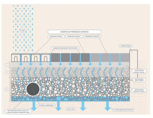
Figure 9. Illustration of a typical permeable pavement system
