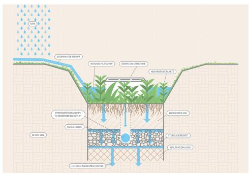
Figure 6. Illustration of a typical bioswale system
